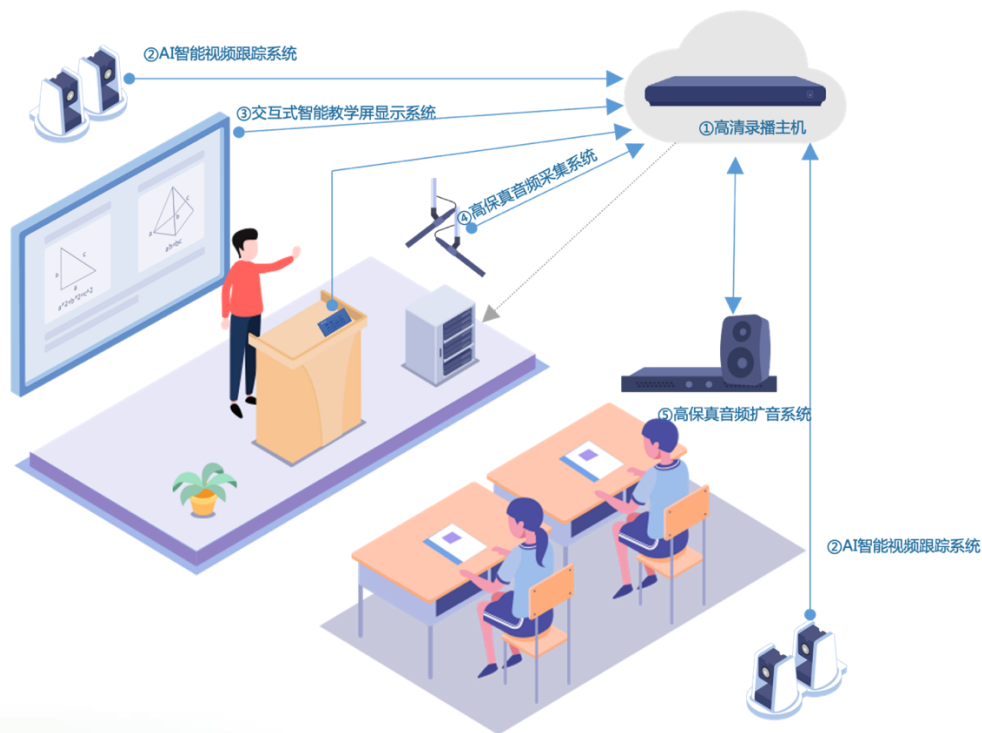
Figure 2 Illustration of the design of high-definition high-quality recording teaching space
